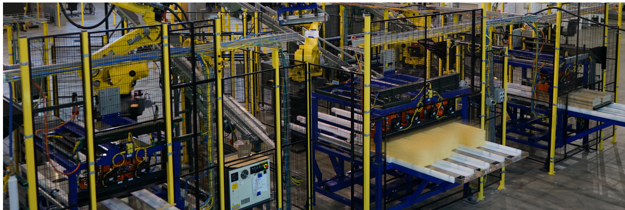
Figure 1: Robotic material handling and custom automation was part of an upgrade for a thermoforming customer in the food and beverage industry. The new automation was to fit between and connected to two existing manufacturing processes on multiple production lines in a 24/7 operation.
