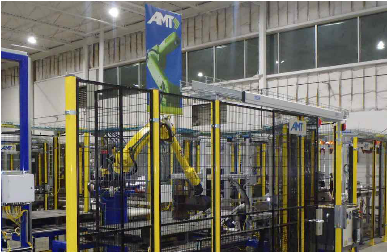
FANUC industrial robot within AMT's automated material handling system for Rehrig Pacific Co.
