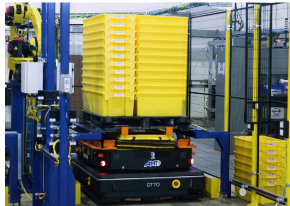
Full AMR leaving front-of-line system.
