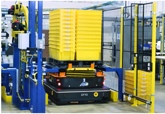
Figure 3: OTTO Motors' autonomous mobile robot efficiently transports stacks of yellow bins, streamlining material handling processes in an industrial setting.
